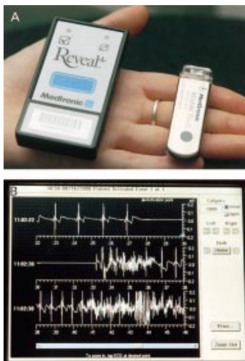
Figure 1. The Reveal Plus monitor (A) is easy to implant and tends to be more acceptable to adolescents than the more traditional non-invasive cardiac event monitors. The Reveal Plus can be activated using an external activator or programmed to recognise and record significant bradycardias, tachycardias or pauses. The quality of ECG recording is usually very good (B). Although there may be some artefact from muscle activity, it is rarely sufficient to affect ECG interpretation.
